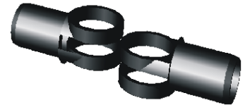
Flexible Coupling - for a variety of hinge actions - 2 double interconnecting rings - flexi-bolt goes through the rings - large end same diameter as standard tube
