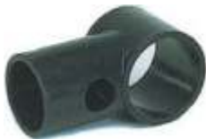
Steering Joint - acts as a 360 degree pivot - standard tube fits through large hole - standard connector end fits into small arm - used for steering shafts - not the same as the 1-hole coupling
